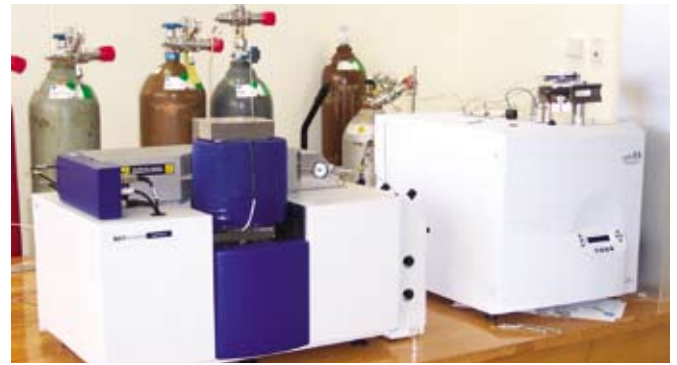
The FAAL's Stable Isotope Ratio Mass Spectrometer
